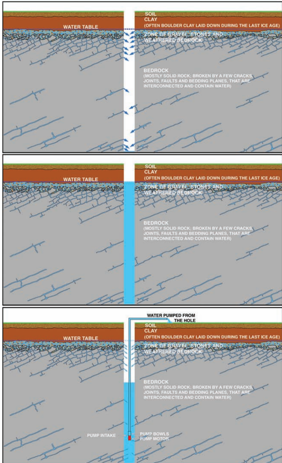
Figure 5. Groundwater flow into a borehole.
