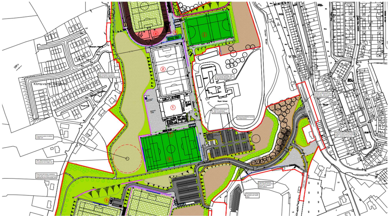
Additional landscaping provided to the south as a buffer between the setting of the school within its own boundary and that of Breffni Stadium (NTS)
