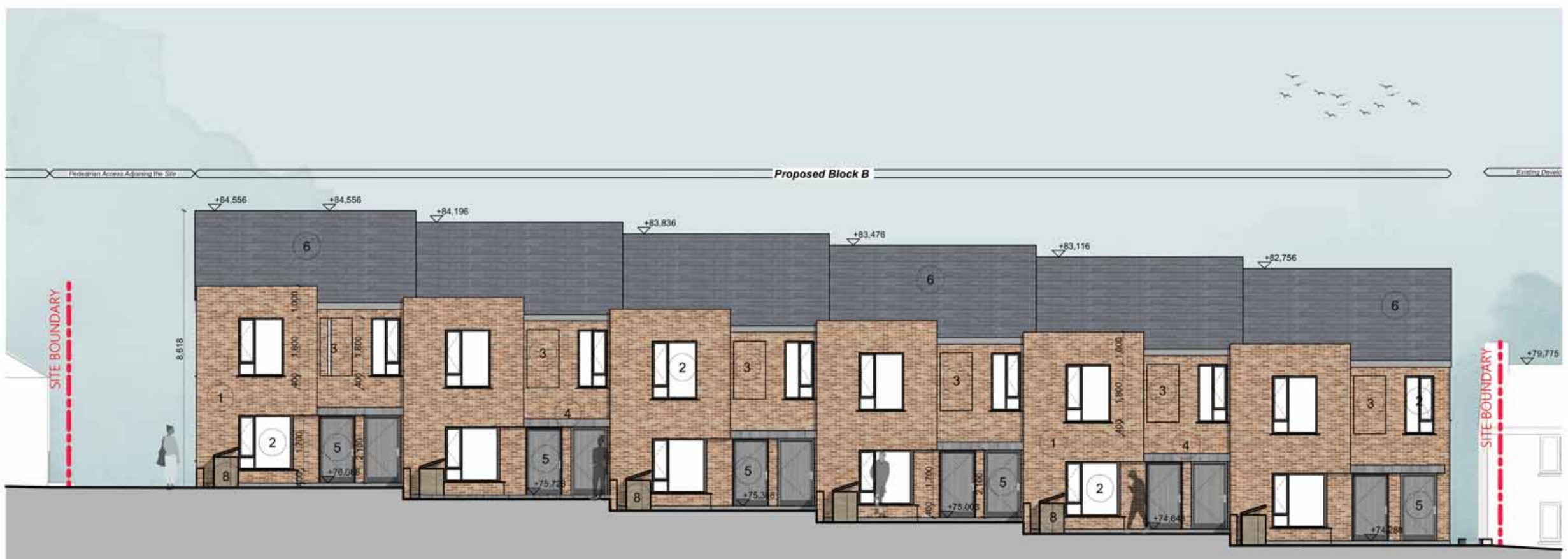
E-07 ELEV-07 Block B Proposed Front Elevation Facing onto St. Brigid's Terrace 1:150
