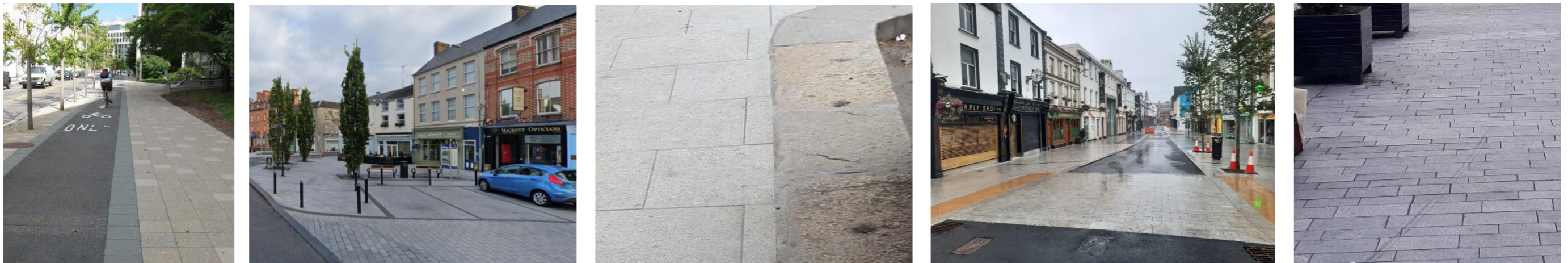
SURFACES : Robust simple materials and patterns - Flagstone footpaths / Setts for square and demarcation lines / pigmented tarmac, ground concrete
