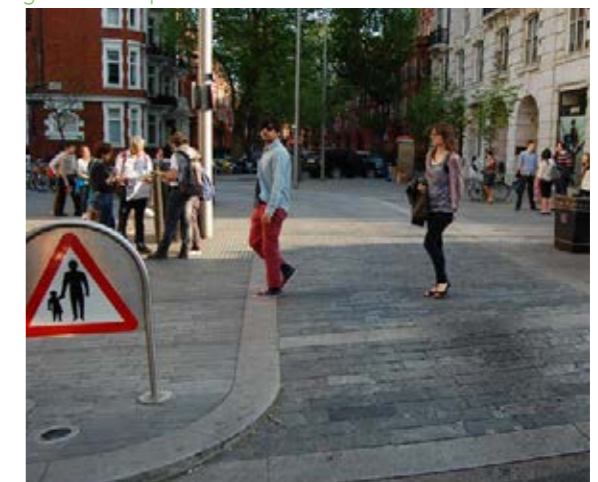
Holbein Place, London. Example of raised traffic platforms & shared surface to street.
