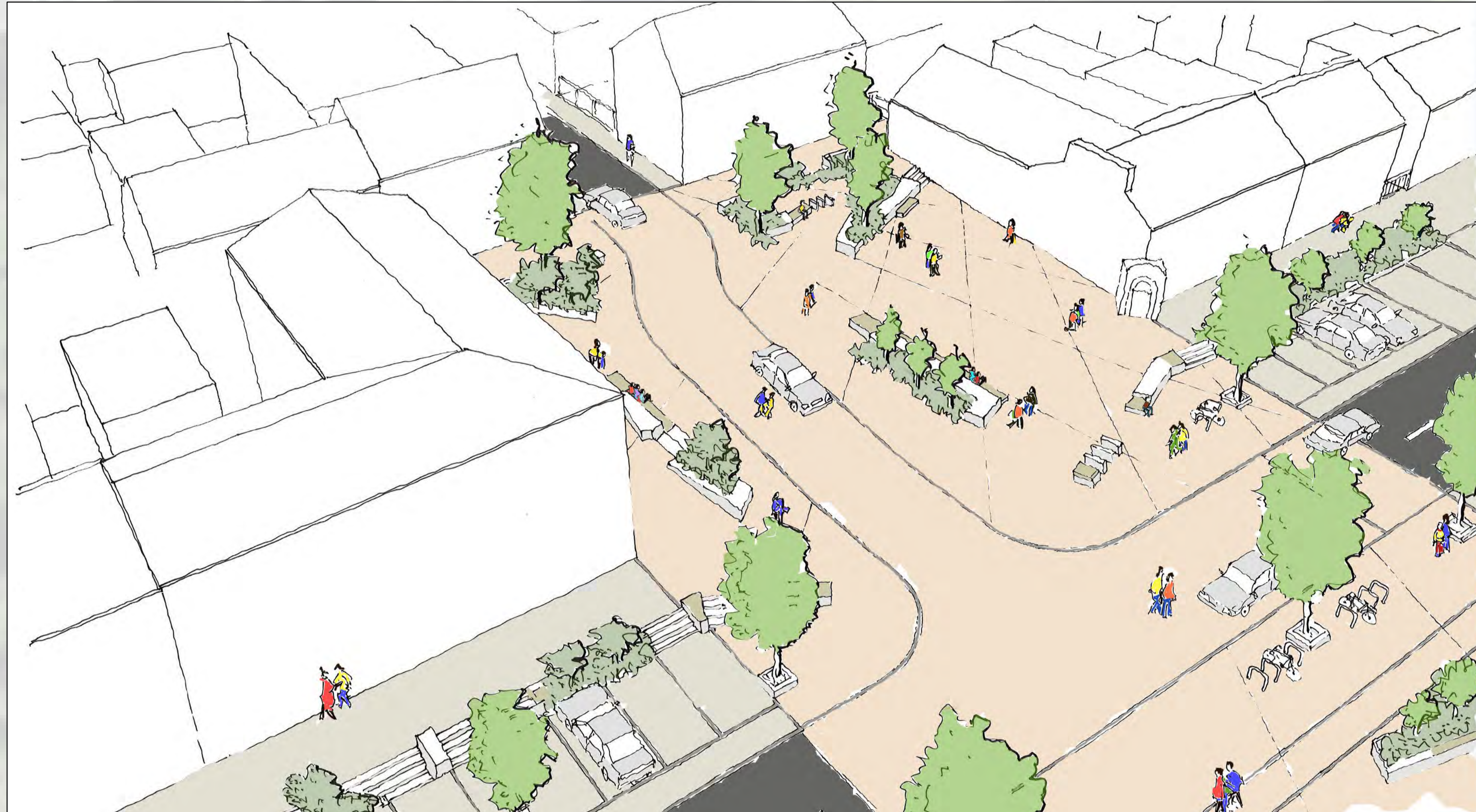
Sketch view of Market Square : Rocks Road is realigned and meets Main Street in a shared space arrangement. Robust high quality paving for markets and other events, steps and ramps are integrated into planters and seating to meet and rest. Please refer to architect's drawing for information on proposed Public Library
