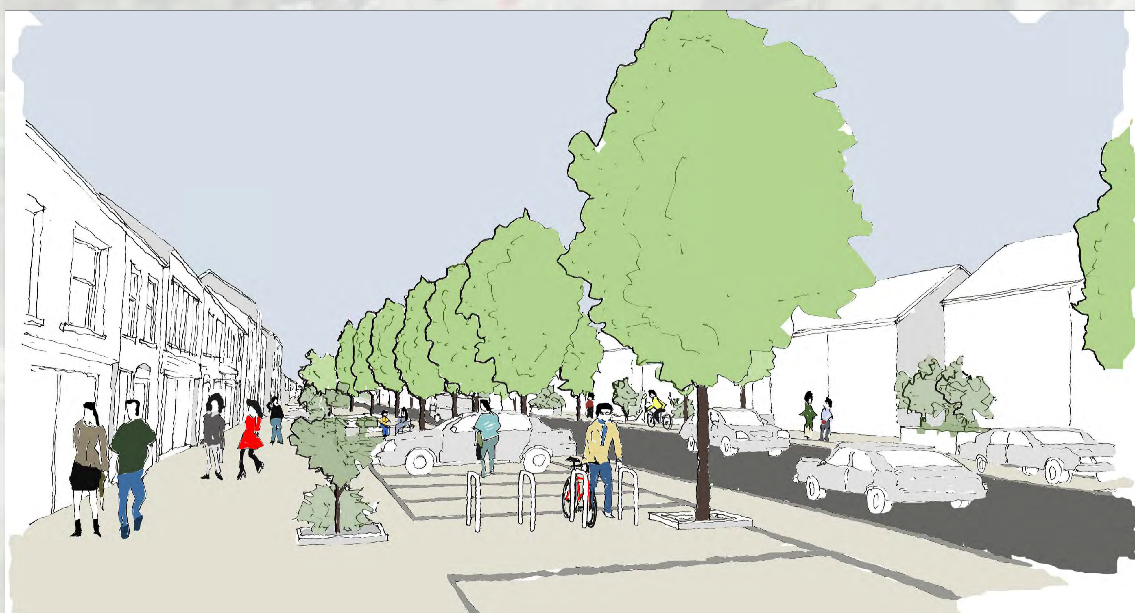
Sketch view of Main Street : Main Street is redesigned as a regular two-way carriageway without median. Parallel parking to the east and perpendicular parking to the west Are integrated into numerous street trees and planters with seating. High quality flagstone paving for generous footpaths and a tarmac two-way cycle lane on the east side.
