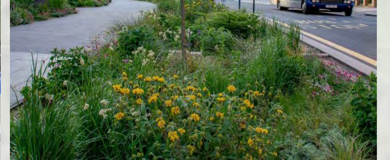
Hard surfaces draining in to soft areas in streets and handstandings – reducing flooding and reproducing natural surface water drainage systems. Soft areas used for mixed native and ornamental planting enhancing ornament and biodiversity.
