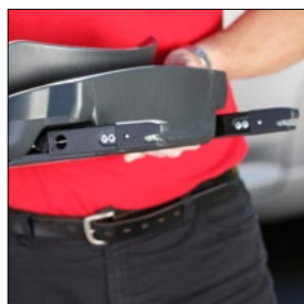
ISOFIX connectors on the child car seat
