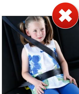
Seatbelt in a dangerous position – booster seat needed
