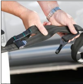
Top tether strap to provide extra restraint and stability
